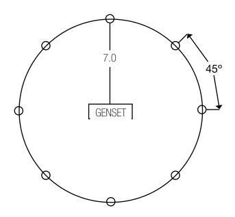
Figure 2 - 7 Meter Measure Points
