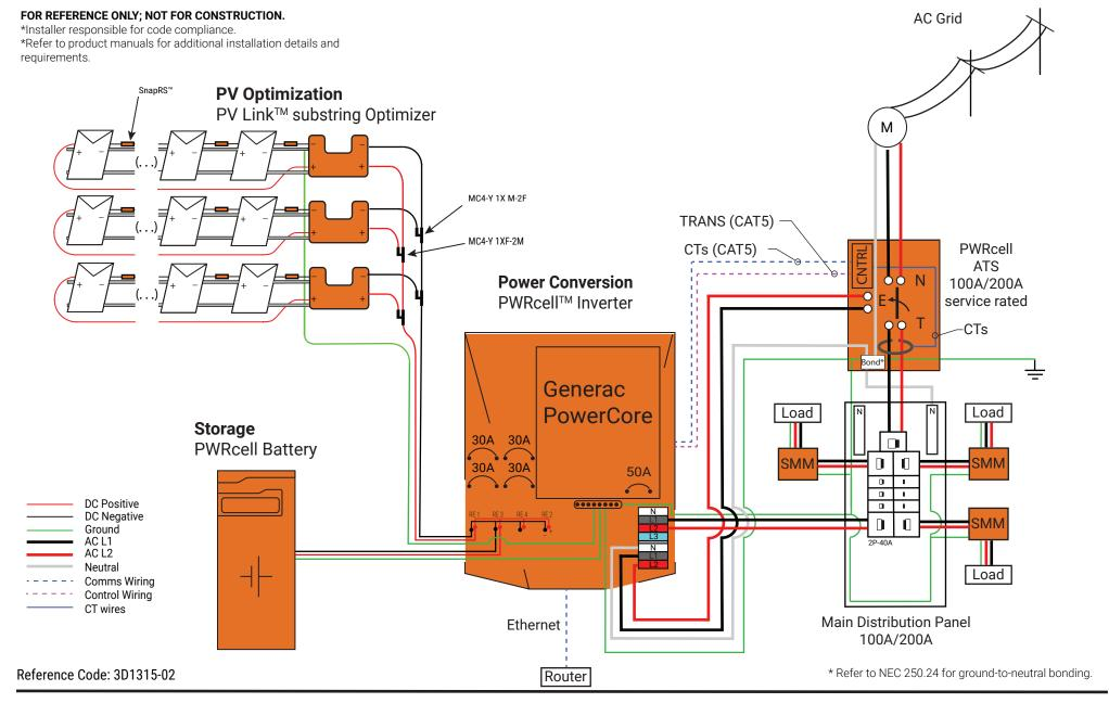
This design shows the Generac PWRcell Whole Home Backup solution. This solution allows for load management capability using Generac SMMs to shed 240V loads as needed.
