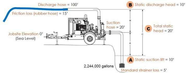
static discharge head. The rate at which you can pump water is referred to as the flow and is often expressed in gallons per minute (GPM). Basically, the higher the vertical distance you are pumping water, the lower the flow or GPM that will be achieved. This is expressed in pump performance curves that will be covered later.
