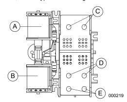
Figure 2-1. Typical Single-Phase ATS Transfer Mechanism
