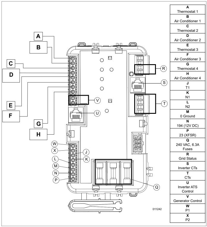
Figure 3-4. Controller Connections
