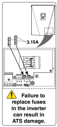
Figure 5-2. Replace Fuses for Generator Integration
