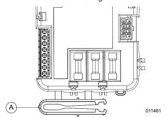
Figure 4-2. Fuse Removal and Installation Tool
