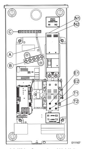
Figure 3-2. Wiring Connections 200 A Unit
