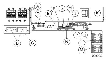
Figure 3-5. Inverter Connections for X7602
