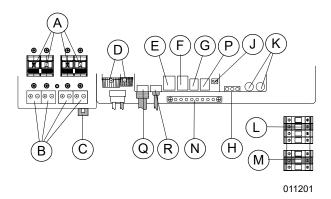
Figure 3-6. Inverter Connections for XVT076A03
