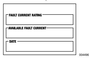
Figure 3-7. Fault Current Label
