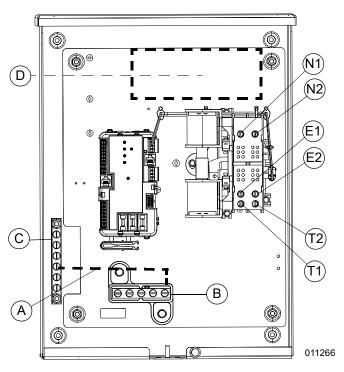
Figure 3-3. Wiring Connections 100 A Unit
